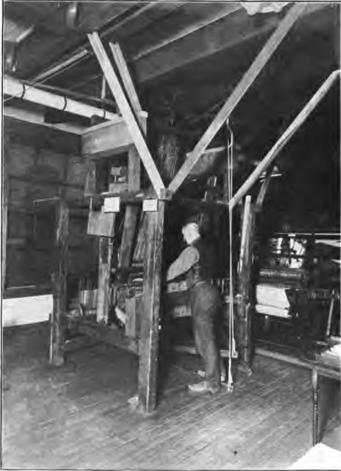
JACQUARD HAND LOOM Weaving Ingrain Carpet at Hull House.
